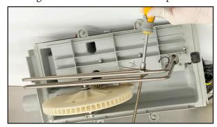
9. Secure the new thermistor with the (2) clamps used to remove the old thermistor.
