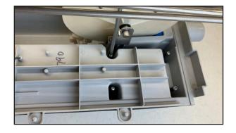
3. Use a Phillips head screwdriver to turn counter-clockwise and remove (5) bolts. Set the bolts aside.
