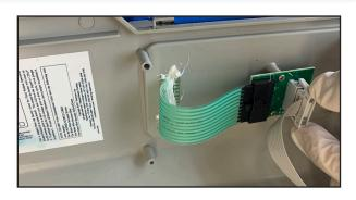
5. Disconnect the push button ribbon from the push button adapter.
