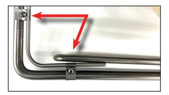
10. Thermistor brackets should be in the position as illustrated above.
