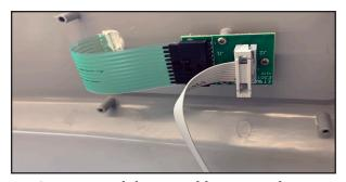
14. Connect push button ribbon to push button adapter on the EECA cover.
