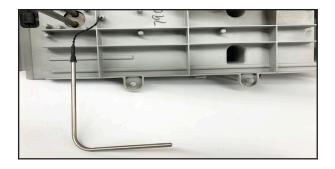
8. Remove the thermistor by pulling out the thermistor thru the bottom side. Set the existing thermistor aside.
