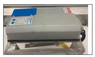
16. EECA cover should be flush with the center module.
