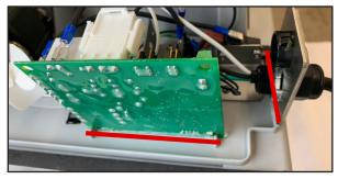
13. Before installing the replacement EECA, be sure the main board and electrical plate are aligned to their holding groove.
