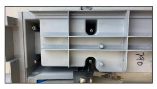
17. Flip the center module and secure the EECA cover. There will be (4) bolts in the front and (1) on the rear.
