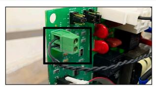
11. Push the Thermistor wires through the center module opening and connect the thermistor wires to the terminals.
