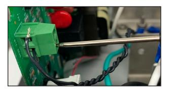
6. The thermistor terminals will be on the rear side of the center module. Using a mini flathead screwdriver, turn counter-clockwise until thermistor wires can be removed.
