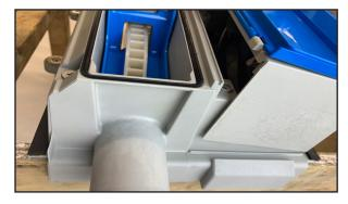
15. With the skimming wheel cover open. Place the replacement EECA on the center module.
