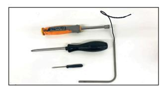
Tools required to replace a PCRAT-3: Phillips head screwdriver, 5/16 nut driver and mini flat head screwdriver.
