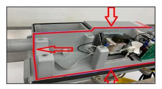
12. Apply the provided sealant along the groove of the EECA cover and center module as illustrated above.
