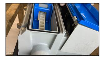
4. Lift the cover over the skimming wheel to pry open the EECA cover. Pull upwards until EECA is completely removed from the center module.
