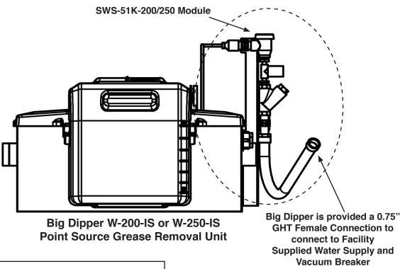
Electrical Requirements\*: 120V, 50/60 Hz, 20 W, 0.5 Amps Water Requirements (Supplied by Facility): 5 Gallons per Hour, 40 - 70 PSI
