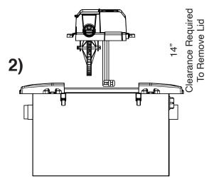
2) Lift the center module up off of the unit, ensuring clearance for the heater.
