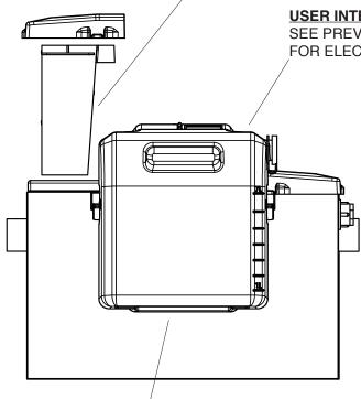
**GREASE/OILS COLLECTION CONTAINER** FOR W-200-IS THROUGH W-500-IS USE PART# GC-10
