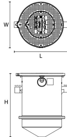
Trapzilla® Solids Separator Models have the same footprint and design as their Trapzilla® Grease Interceptor counterparts of like liquid capacity, making installation of additional units easy!
