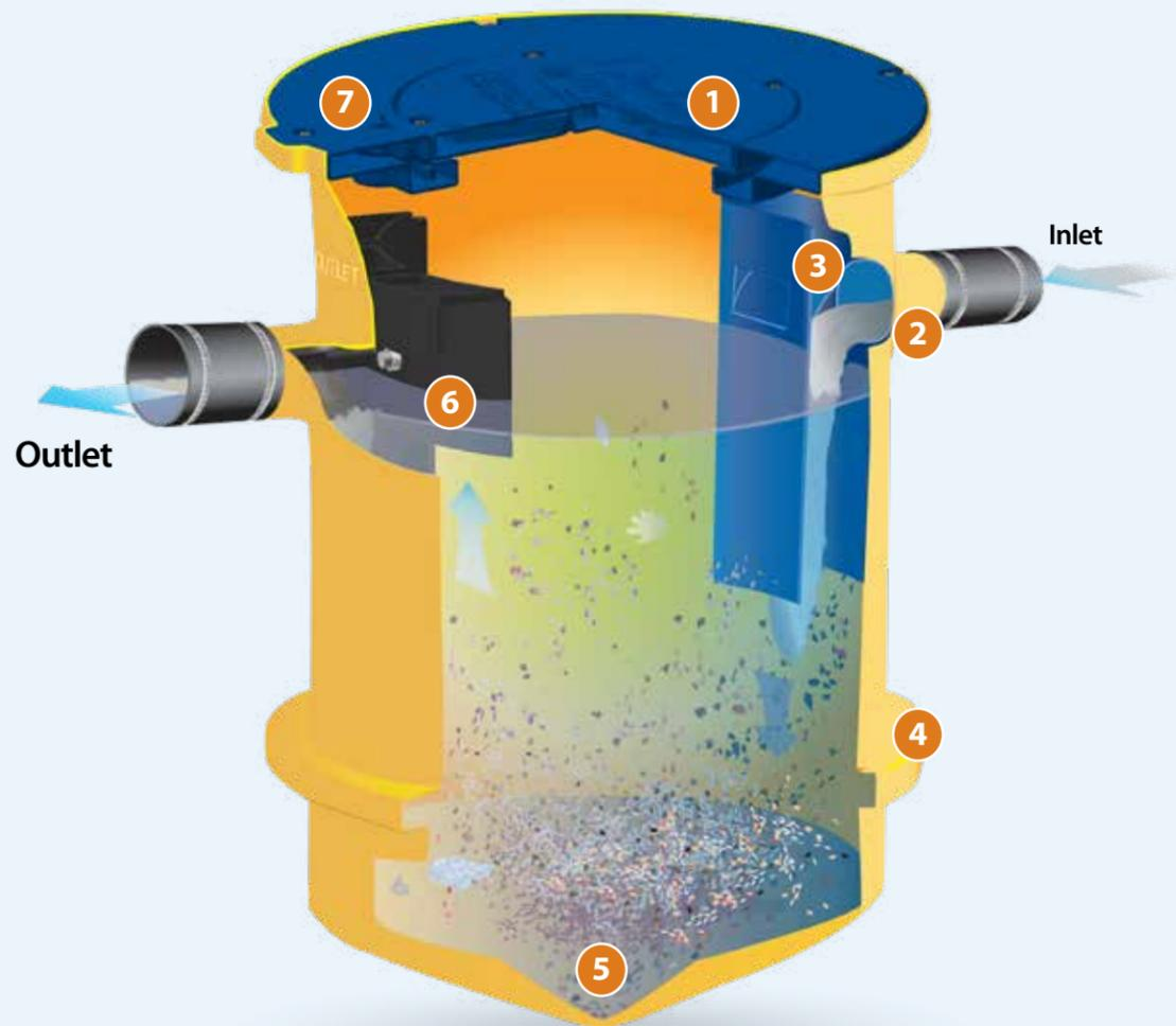
Solids-laden effluent from the kitchen flow is slowed and forced downward in a vertical baffle, where solids filter out of the flow and sink to the bottom of the solids storage area. The “cleaned” effluent flows through the outlet. Pumping the Trapzilla® Solids Separator is easy—the pumper removes the lid and vacuums out the solids.
