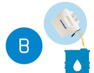
Uncap and empty the grease collector into an approved waste container
