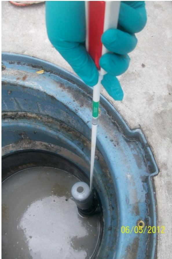
1,000 mL Container Used to Collect Wastewater Samples from the Trapzilla®
