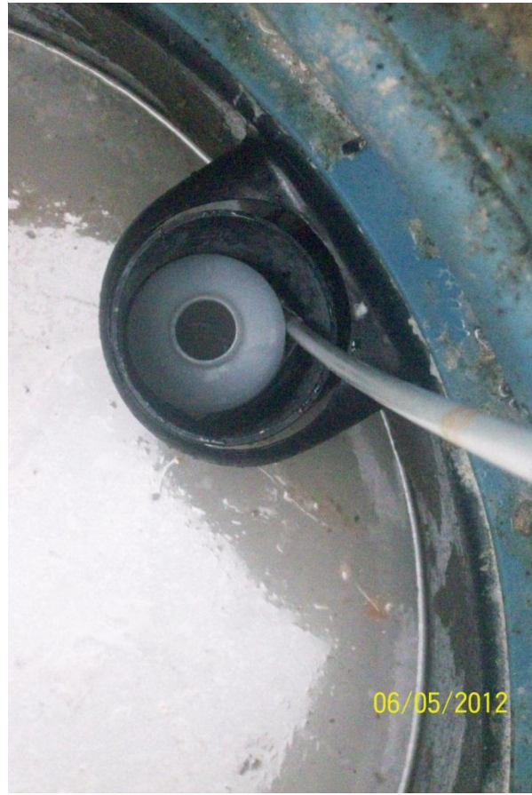
1,000 mL Container Submerged in the Trapzilla® Effluent Pipe
