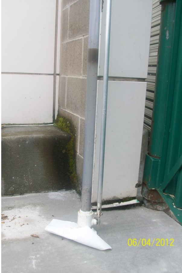
Dip Stick Probe Used to Verify the Pumping Frequency
