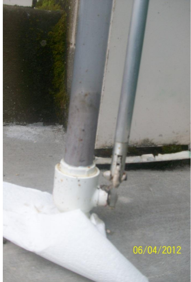
Level of Solids Accumulated at the Bottom of the Dip Stick Probe
