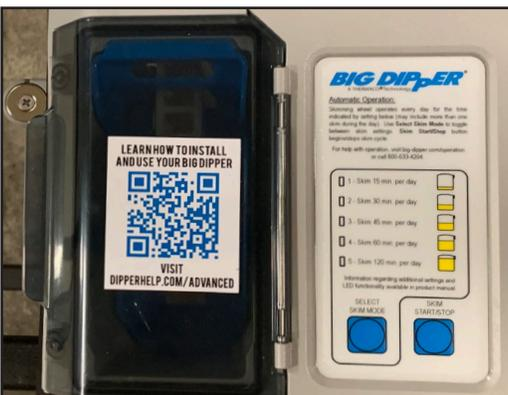
4. Close the new flip door. You should now be able to open and close the flip door to access the wiper blade for weekly maintenance.
