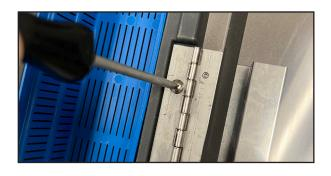
Screw the support bracket and lid hinge to the Dry Strainer on the side nearest the Big Dipper.
