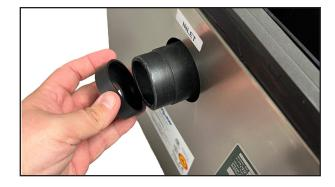
Remove the Flow Control from the Big Dipper Inlet.
