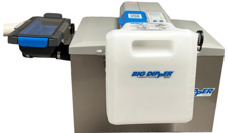
The Big Dipper<sup>®</sup> DSA-25-1 Dry Strainer separates and collects coarse solids such as rice, coleslaw, and other food scraps larger than 0.065 inches (1.59 mm) in diameter. The removable tray allows for easy and sanitary disposal of the collected solids directly into a trash receptacle. The Dry Strainer is made of durable plastic and offers a convenient solution for waste disposal of coarse solids.
