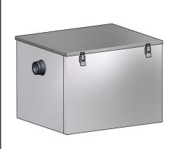
The Big Dipper Passive system is a passive Hydromechanical Grease Interceptor. As greasy kitchen effluent drains from kitchen fixtures, the unit captures the free-floating grease & oils. Only the "cleaned" water exits the unit and flows into the facility drain lines. Point Source Big Dipper Passive units operate most efficiently when sevicing single fixtures such as a 1 to 4-compartment sink or a pre-rinse station. Centralized Big Dipper Passive models can be used to handle entire kitchen flows.
