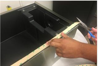
8. With residue removed, lay new gasket on front edge of unit and cut to length. Do NOT stretch gasket.
