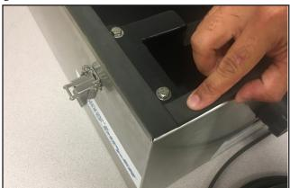
10. Repeat measuring and placing new gasket on the back, then sides of tank. Do NOT overlap gasket at corners!
