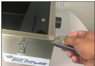
4. Remove the gasket by using a razor blade, paint scraper, or other sharp item.
