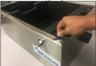
5. Starting at one corner, remove gasket by slowly pulling upwards and scraping residue with blade.
