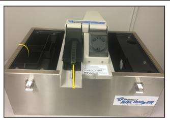
2. Unlatch and remove Inlet/Outlet covers and Electrical Assembly from Big Dipper Tank
