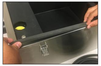
9. Remove tape from adhesive underside of gasket and apply adhesive side down to the top of the front edge of unit.
