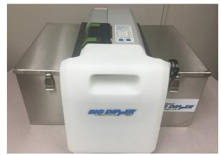
16. Connect the unit to a power source. Follow instructions found in the instruction manual or on www.big-dipper.com to set correct skimming mode and time.
