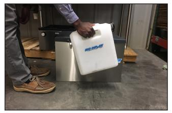
15. Place grease collector on unit by aligning the grease collector with the opening on the unit and turn the collector slightly clockwise to lock into position.
