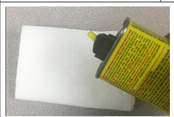
7. Remove remaining residue with an adhesive remover and a clean rag. Acetone works best.
