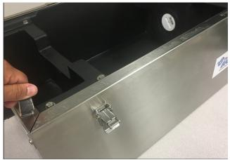
6. Repeat this process with all sides until the gasket is removed. Some residue may remain.
